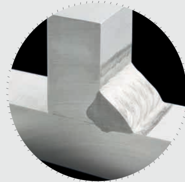
/ Optimal weld face profile and toe transition
