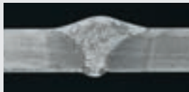
/ Stick-out 15 mm V_{wire} = 10 \text{ m/min} I: 300 - 250 \text{ A} Steel 6 mm
