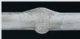
/ Stick-out 15 mm V_{wire} = 10 - 13 \text{ m/min} I: 300 \text{ A} Steel 6 mm
