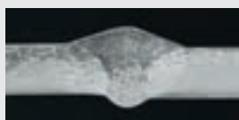
/ Stick-out 30 mm V_{wire} = 10 - 13 \text{ m/min} I: 300 \text{ A} Steel 6 mm
