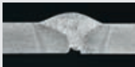
/ Stick-out 30 mm V_{wire} = 10 \text{ m/min} I: 300 - 250 \text{ A} Steel 6 mm
