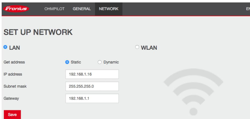
The screenshot shows the 'SET UP NETWORK' page in the Fronius Ohmpilot web interface. The 'LAN' tab is active, and the 'Static' radio button is selected under 'Get address'. The IP address field contains '192.168.1.16', the Subnet mask field contains '255.255.255.0', and the Gateway field contains '192.168.1.1'. A red 'Save' button is located at the bottom left. A large, faint Wi-Fi symbol is visible in the background on the right side of the page.
